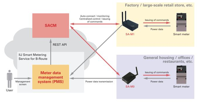
Figure 2: Linking with the IIJ Smart Metering Service for B-Route
